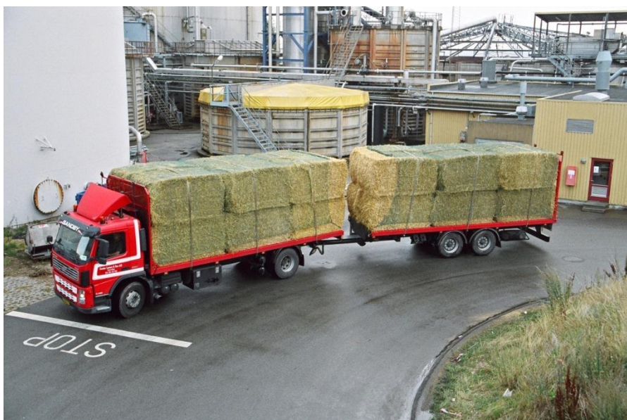
Fig. 10: Normal transport of straw for large scale energy use. There are 24 big bales in two layers on the truck and trailer, with a total weight of 12 tons. Unloading takes place with an automatic crane taking 12 bales in one lift. Weight of the bales and water content is measured during the unloading process.
