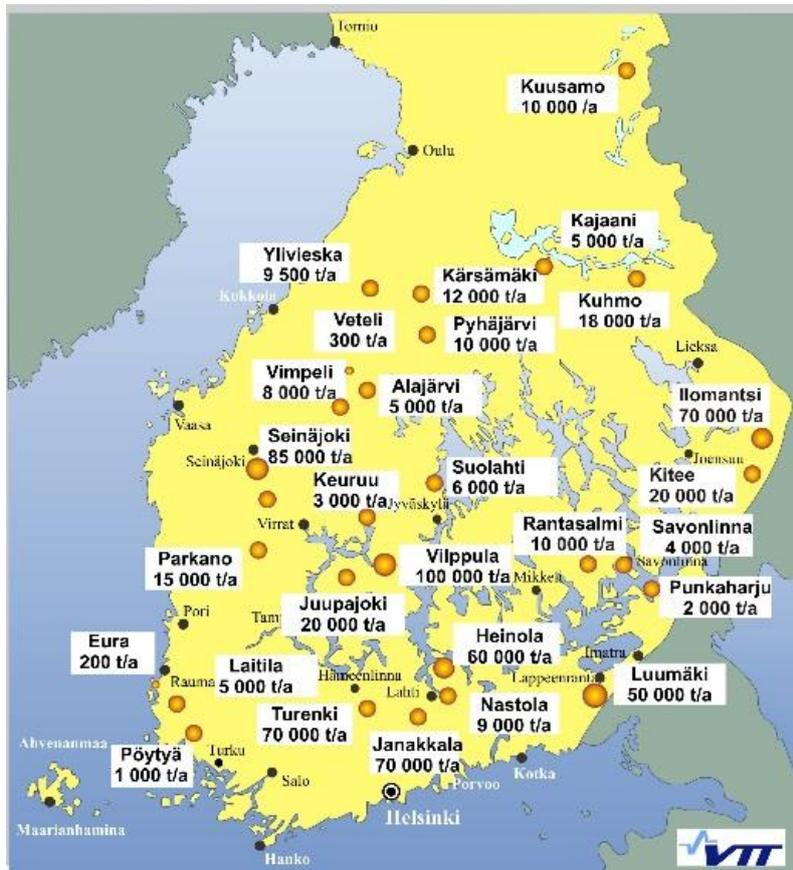
**Figure 3.29 - Location of wood pellet production plants and their capacities in tonnes in Finland, in 2014 (Karhunen A. et al., 2014).**
