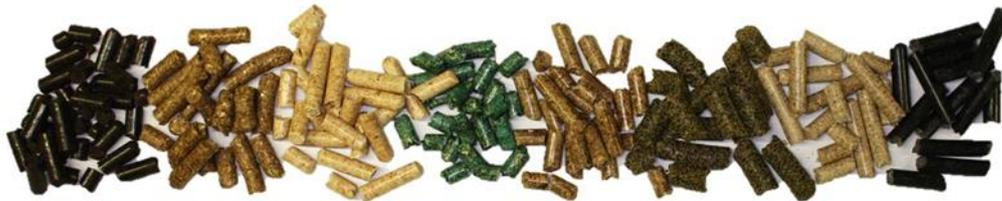
**Figure 1.1 - Pellets examples from different materials and processes (source: DBFZ)**
